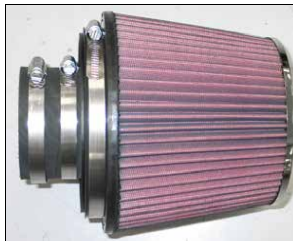
15. Install the silicone hose (08698) onto the filter adapter and secure with the provided hose clamp.
