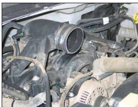
13. Install the provided silicone hose (08698) onto the intake plenum and secure with the provided hose clamp.
