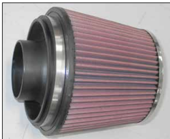
14. Install the filter adapter into the K&N® air filter and secure with the provided hose clamp.
