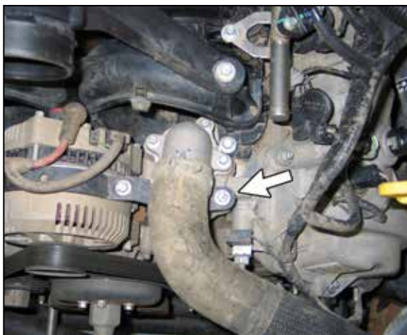
7. Remove the upper alternator mounting bolt shown. NOTE: This bolt will be reused in the next step.
