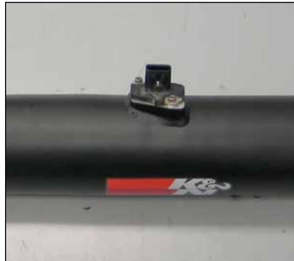
18. Install the mass air sensor into the K&N® intake tube and secure with the provided mounting screws.
