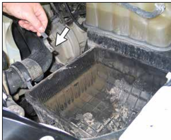
11. Remove the center air box lid mounting clip from the lower air box as shown.
