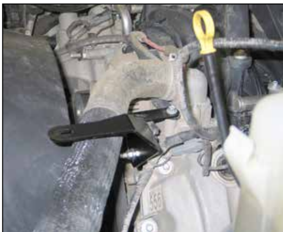
8. Install the tube mounting bracket (083111) and secure with the provided hardware and the bolt removed in the previous step.
