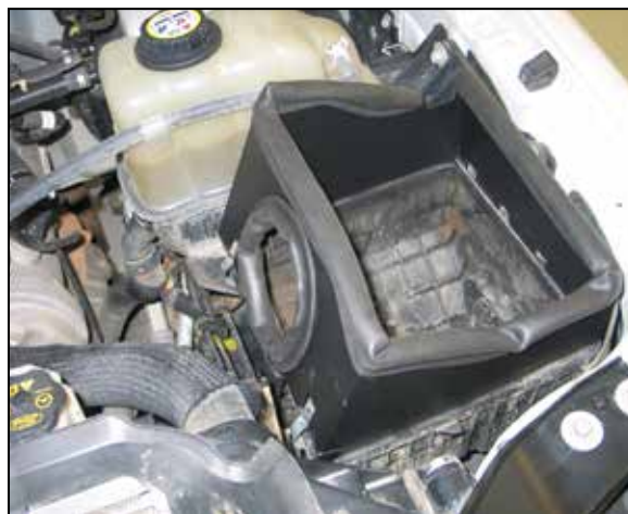
12. Install the heat shield assembly onto the lower air box and clip into place with the upper air box mounting clips. NOTE: A gap is normal between the lower air box and heat shield on the clip side of the heat shield.
