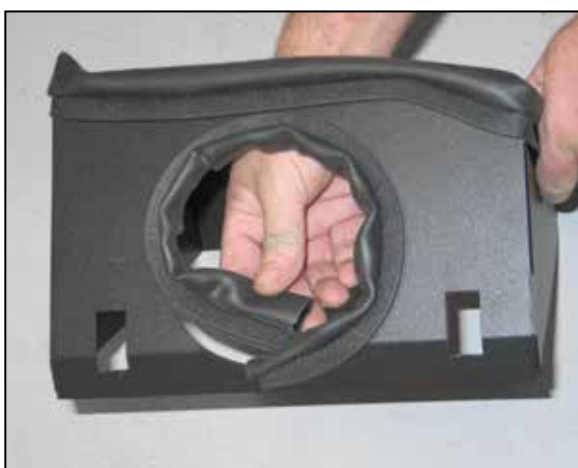
10. Install the provided edge trim into the hole in the heat shield as shown. NOTE: Some trimming of the edge trim will be necessary.
