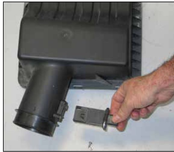
17. Remove the two screws securing the mass air sensor to the upper air box and then remove the mass air sensor from the upper air box.
