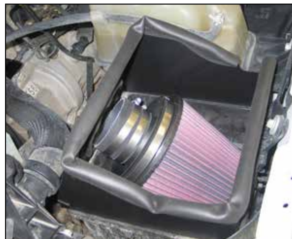
16. Place the filter assembly into the lower air box housing as shown.
